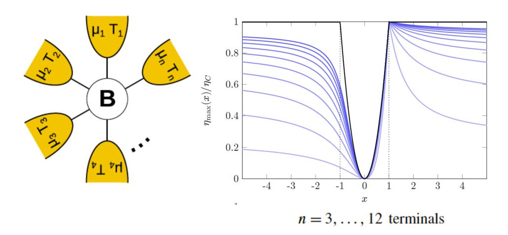
Numerical evidence that the power vanishes when the Carnot efficiency is approached
